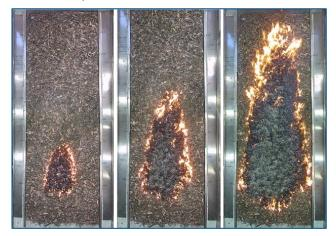
Figure 3. Rectified overhead video frames of an experimental fire. From left to right: 2, 4 and 6 minutes since ignition from a 400-mm-wide line, wind speed 2 m/s, FMC 5%.
